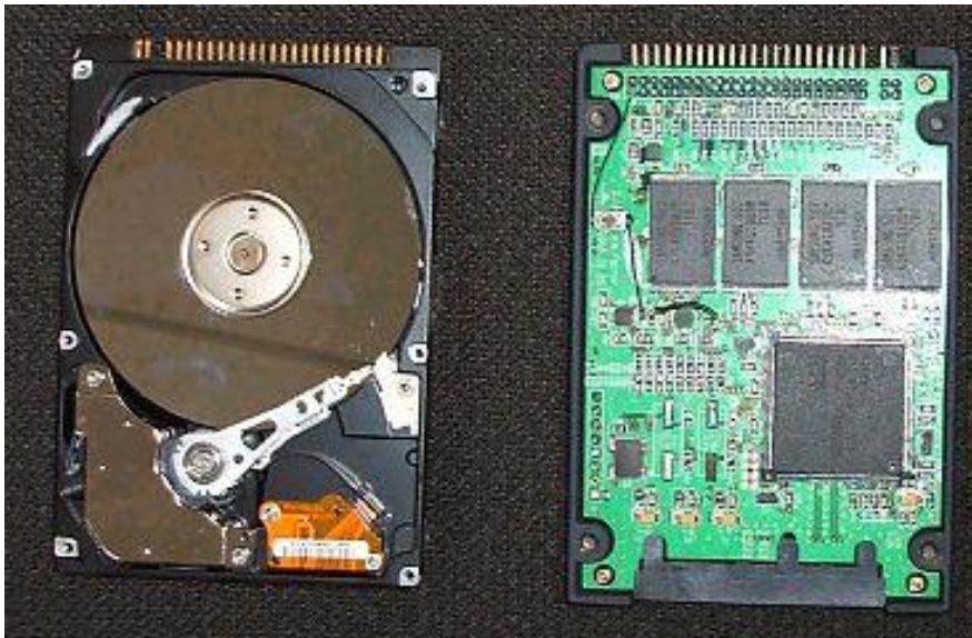
2.5" HDD Flash SSD (101x70x9.3mm)
