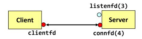
3. Server returns connfd from accept. Client returns from connect. Connection is now established between clientfd and connfd.
